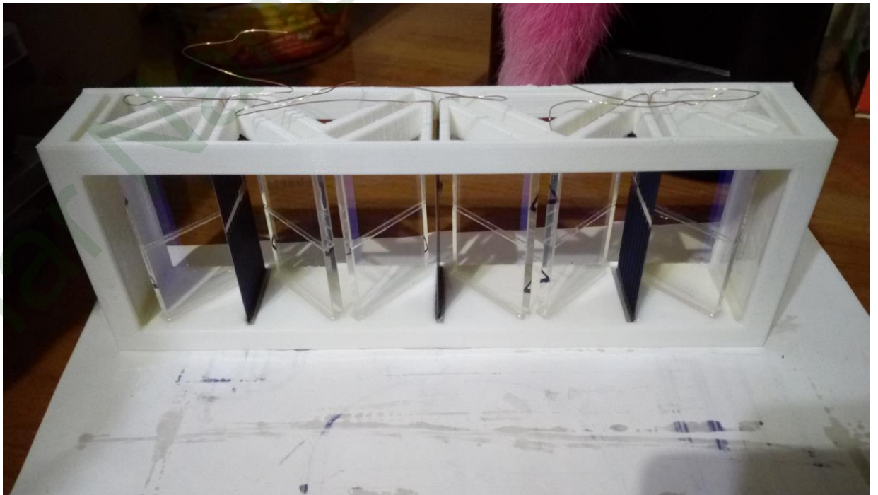
Figure 6. Solar window with double sided solar cell
